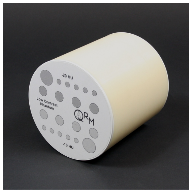
2DL with different contrast cylinders of -10 HU and -20 HU!
